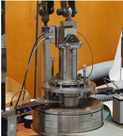
Figure 1. Modified fragmentation rheometer apparatus
